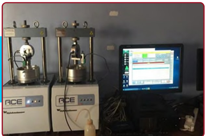
Automated Consolidation Test Equipment for consolidation testing.
